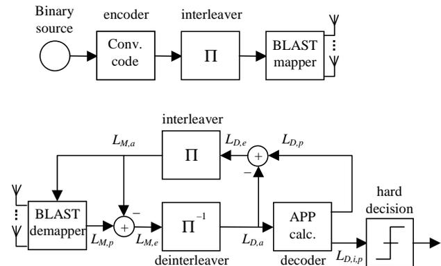
Figure 1: Turbo-BLAST system configuration.
