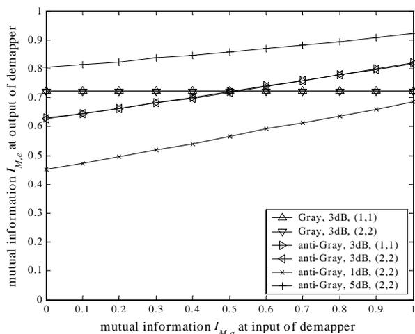
**Figure 3: EXIT characteristics of QPSK BLAST demapper operating in AWGN for different mappings,  $E_b/N_0$  (at code rate 1:2) and  $(N_t, N_r)$ .**
