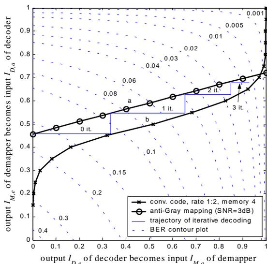
**Figure 5: Simulated EXIT characteristics and real trajectory of iterative decoding for QPSK, anti-Gray mapping,  $E_b/N_0 = 3\text{dB}$ , rate  $\frac{1}{2}$  memory 4 code and  $(N_r, N_t) = (2, 2)$ .**
