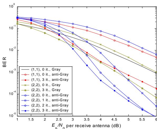
**Figure 6: BER performance a Rayleigh flat-fading channel for QPSK, rate  $\frac{1}{2}$  memory 4 code, different mappings and antenna configurations.**
