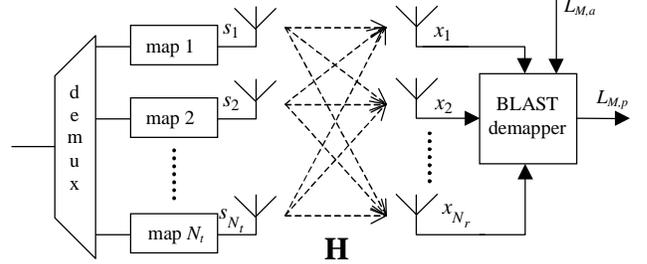
Figure 2: The physical model of a BLAST communication channel.
